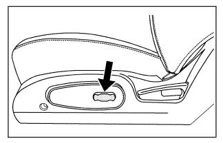
If your vehicle has this feature, the control is located on the outboard side of the driver's seat. To adjust the seat do any of the following:
